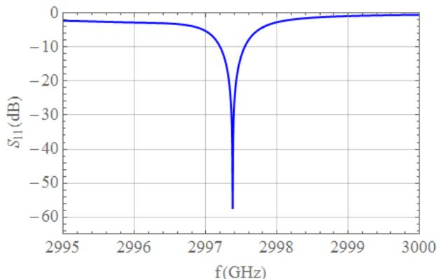
Figure 10: Measured  $S_{11}$  spectrum of a tuned module.
