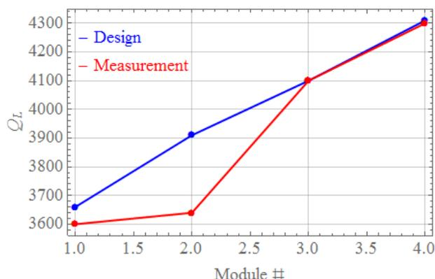
Figure 8: A comparison of simulated and measured  $Q_L$ .
