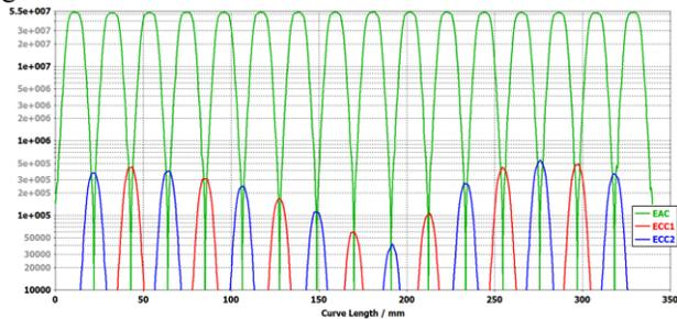
Figure 3: Accelerating and coupling cell fields in a tank.
