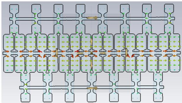
Figure 4: RF design of a tank showing accelerating field.
