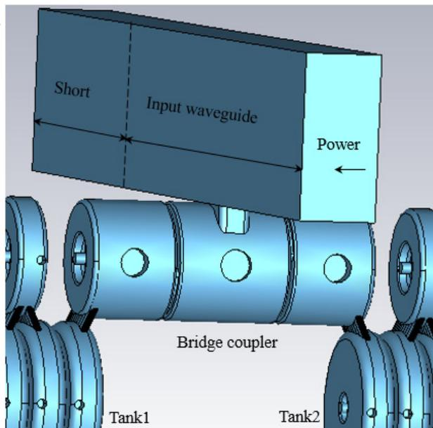
Figure 5: Bridge coupler RF design.
