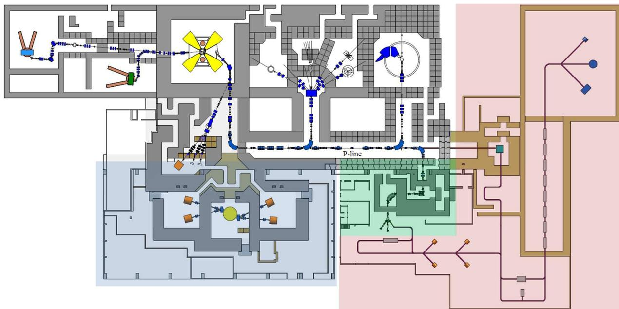
Figure 1: Layout of the main facility at iThemba LABS, with ACE Isotopes (shaded blue), LERIB (green), and the second phase of ACE Beams (pink).
