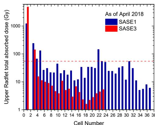
Figure 5: Total absorbed doses in logarithmic scale for SASE1 and SASE3 after the first year of operation.
